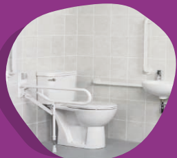
No contrast e.g. white on white is difficult to see and use
